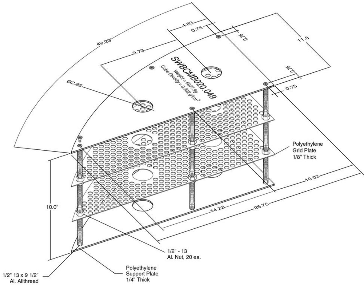
Figure F-3. End type SWB matrix module.
