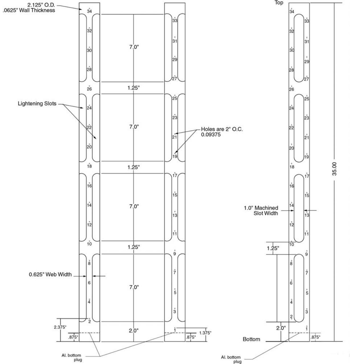
Figure F-4. SWB matrix surrogate PDP standard insert fixture.
