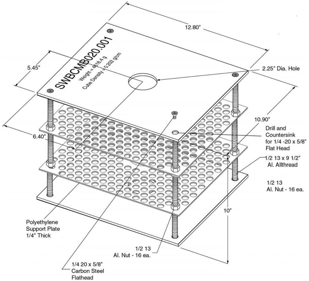
Figure F-2. Center type SWB matrix module.
